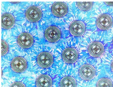
FIGURE – Silicon carbide fibres in a titanium matrix (© ONERA)
