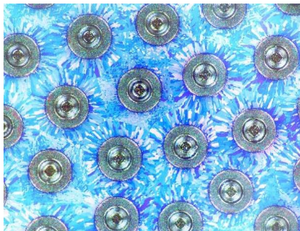
(a) Silicon carbide fibres in a titanium matrix (© ONERA)
